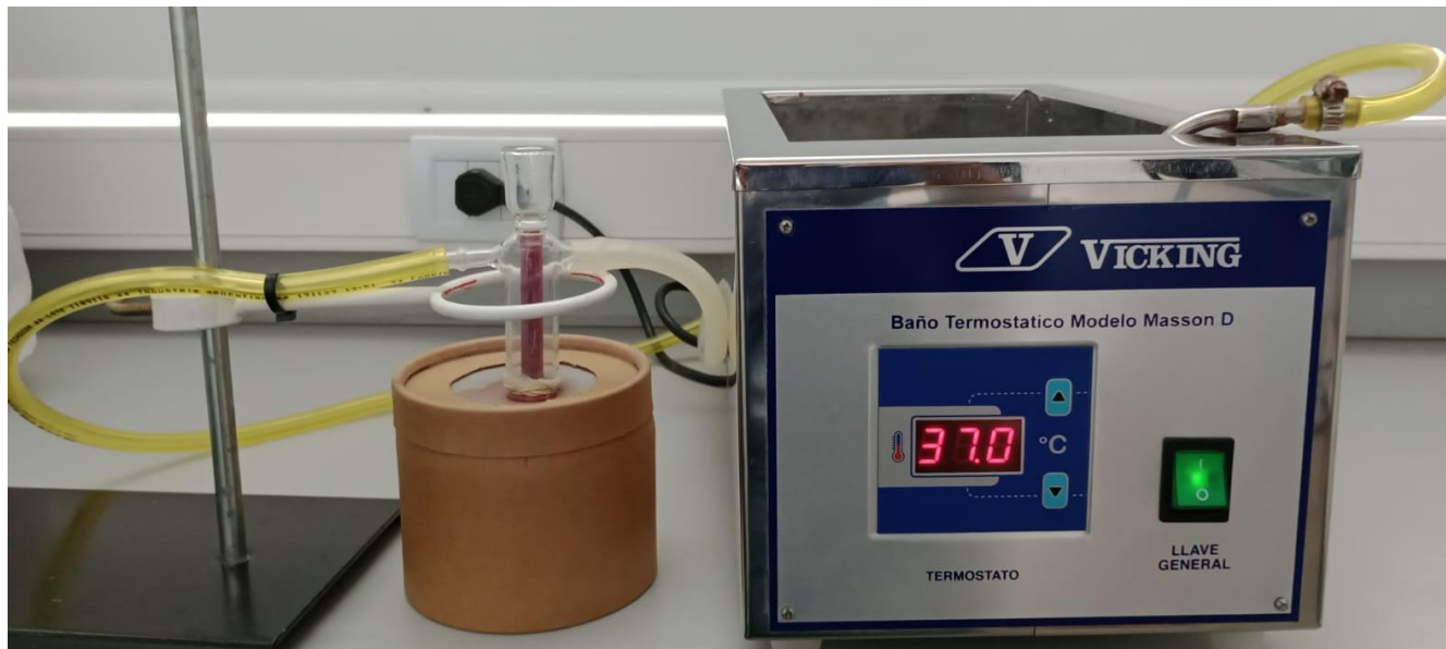
Fig. 1. Artificial feeder. The glass feeder evaluated simulates natural feeding. It employs cattle gut membrane that mimics human skin, it has a capacity of 5-6 ml, the temperature is regulated in order to keep the blood at 37 °C through a thermostatic circulator bath, and it employs human blood with sucrose as meal source.
